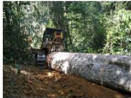
d. Bulldozer skidding tree-length timber along skid trail towards nearest matau
