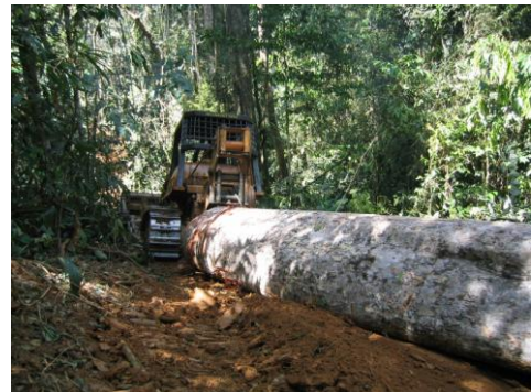
d. Bulldozer skidding tree-length timber along skid trail toward nearest matau
