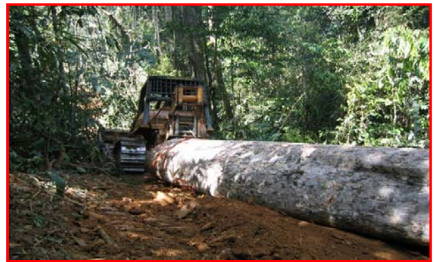
d. Bulldozer skidding tree-length timber along skid trail towards nearest matau
